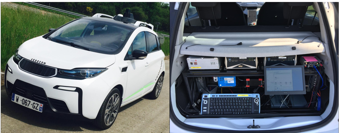
Figure 3: VEDECOM demonstrator: installed sensors and intern hardware platform.
